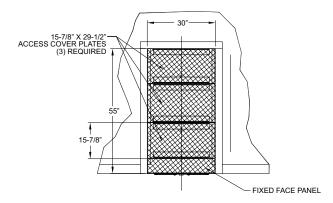
PIT MOUNTED VEHICLE RESTRAINT & COVERS TOP VIEW
